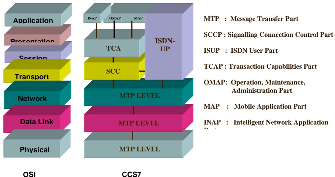
**Figure A:** The OSI Reference Model and the SS7 Protocol Stack
