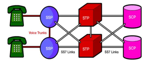
Figure 1: SS7 Signalling Points
