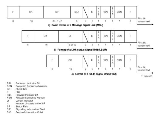
Figure 2: Signal unit format
