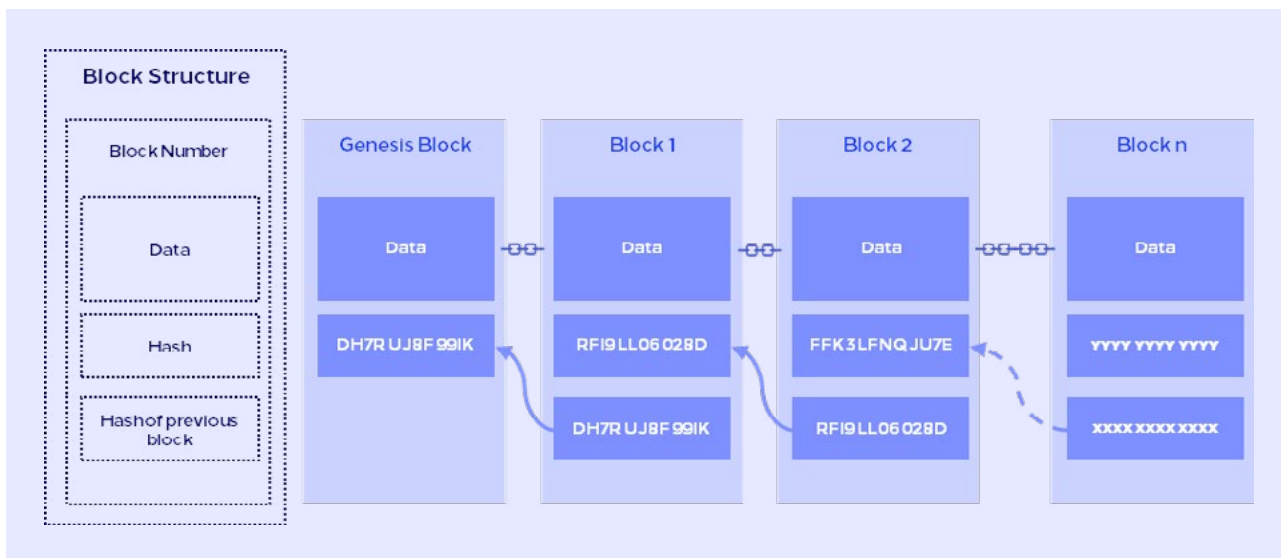
Figure 2: Chain of blocks in a Blockchain linked by a hash of the previous block
